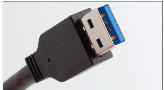
↑ USB 3.0 connectors look and act in the same way as their USB 2.0 predecessors. But the internal spec means connectivity speeds are quicker
